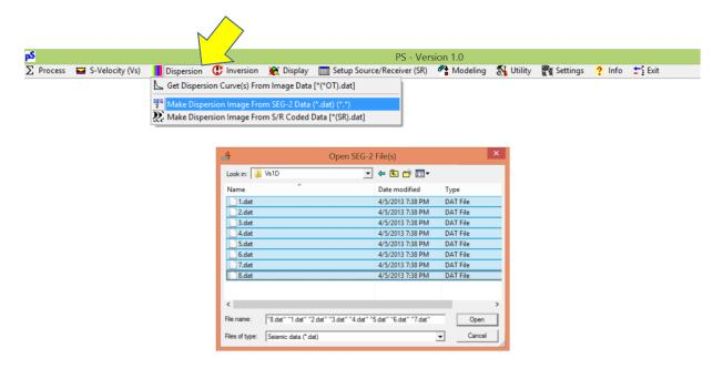
To import a data set of field records already in PS format with a proper source/receiver (SR) configuration encoded, go to "Dispersion"  $\rightarrow$  "Make Dispersion Image From S/R Coded Data" and then select one file.
