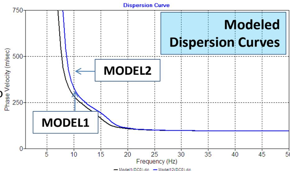
The graphs indicate it is critical to acquire surface waves lower than 20 Hz so that the two dispersion curves can be discriminated and the target zone can be detected if data acquisition and processing are successful.
